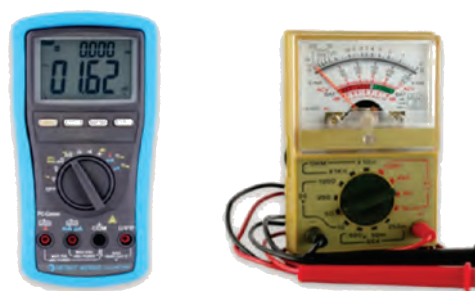
Fig. 16.3: Comparison of digital and analog ammeters
