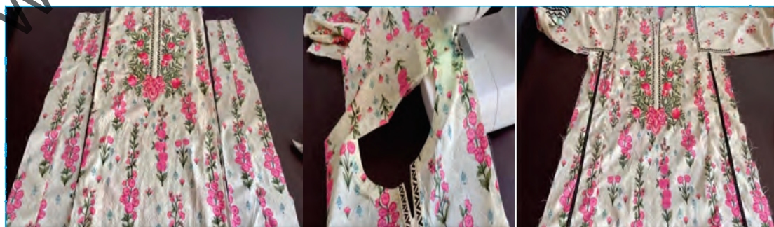
Figure 10.4.1.4: Side Panel (Kali) with Sleeve Attachment
