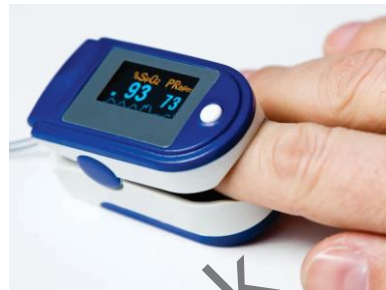
Figure 10.2: Use of Pulse Oximeter
